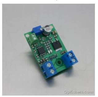
This is an advanced TEC controller using a microprocessor unit.
