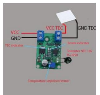
TECs can be connected parallel or in series. Please remember that high current needs proper wiring with bigger cross section of the cables.
