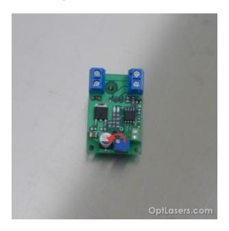
3. Next, slowly rotate the potentiometer clockwise until the blue LED lights up, which means that TEC is running and temperature is decreasing. After reaching the desired temperature turn the potentiometer a little counterclockwise in order to make the blue
