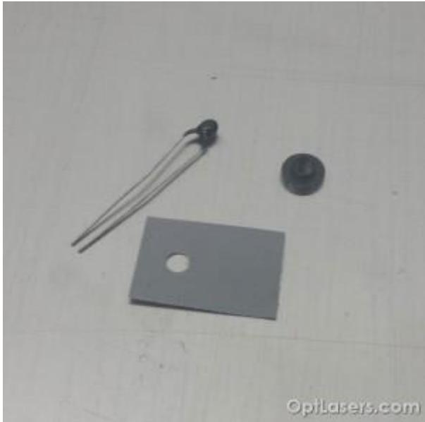
The driver has a temperature sensor connector. It is recommended to use a NTC 10k sensor.
