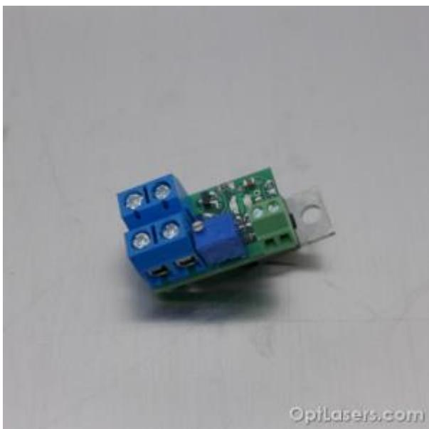
Tiny size and big operating currents make it possible to use this driver in almost any project. Temperature stabilization reaches  $\pm 0.4$  degrees Celsius accuracy. High current, wide voltage range and high accuracy in a device of only 16.5 x 25.5mm in size! The driver works in a cooling mode and uses voltage feedback from a 10k NTC thermistor.
