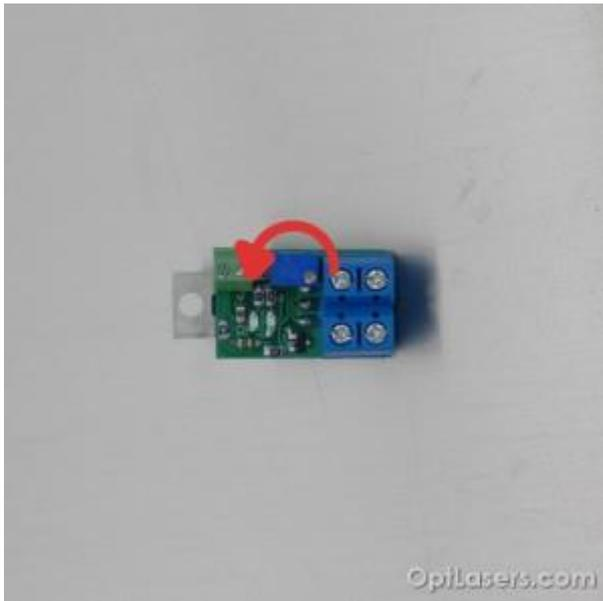
3. Next, slowly rotate the potentiometer clockwise until the blue LED lights up, which means that TEC is running and temperature is decreasing. After reaching the desired temperature turn the potentiometer a little counterclockwise in order to make the blue LED off. By doing so, you can achieve a state of temperature balance. Exact temperature can be read thanks to a temperature sensor with a display or a pyrometer.
