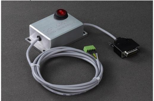
e) Insert the female D-Sub connector on the adapter cable into the male socket on the Stepcraft machine:
