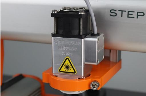
d) Locate the Stepcraft PLH3D-6W Adapter, which will be used to connect the laser head to the Stepcraft machine:
