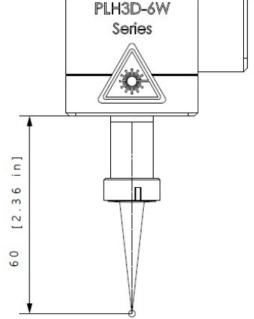
the Beam Cone Shape of the PLH3D-6W-XF Laser Head
