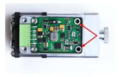
4. Use a small flat screwdriver to move the switch into second position (marked "ON"). See image for the reference. Now the laser head's Modulation Input #1 accepts voltage range 0 - 10V.
