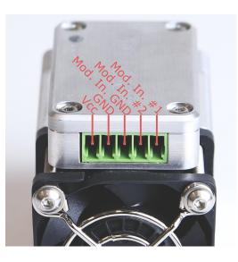
PLH3D-6W-Series Laser Head Pinout:
