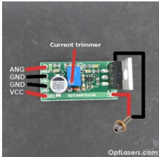
**Note! When power supply is turned on or turned off, the signal ANG must be low.**
