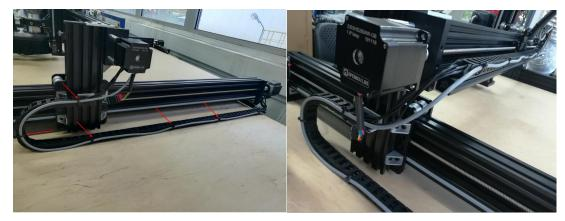
For the users who prefer to put the cable through the drag chain, bear in mind that you will have to remove one of the end connectors in the PLH3D-CNC Adapter to Laser Head Cable. Also, remember that the 5 wires' connection is mirrored on the opposite side of the cable (and, thus, the order of the wires is flipped).
