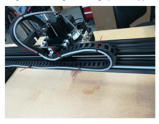
4. For the next step, pass the cable around the X-axis motor and then secure the cable along the Y-axis drag chain in a similar fashion as in the previous step.
