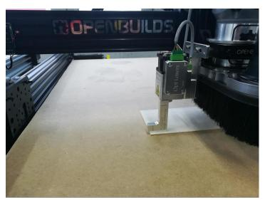
3. Attach the nozzle to the laser head using their natural magnetic attraction. Adjust the length of the nozzle by loosening the screw as shown in the picture below. The distance between the nozzle and the surface of the material being engraved should be around 5-8 mm.
