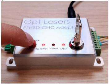
7. To save the current setting, wait five seconds with the button released. To quit without saving, turn the key switch off before five seconds elapse.
