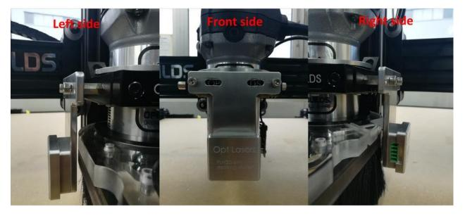
• For mounting the docking station on the front side you have to remove the dust shoe. There is no risk that the laser head would collide with machine parts.
