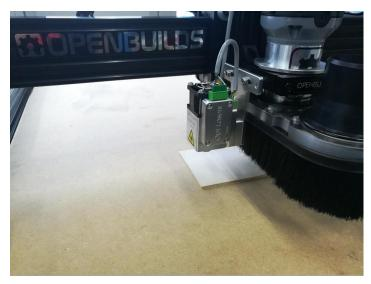
2. Using the PLH3D-6W Height Reference Tool, position the laser head 60 mm above the plywood specimen's surface.
