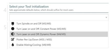
8. In the subsequent section of the machine configuration, you can set customized parameters for the machine working area and laser power. Furthermore, it also shows the G-code commands and settings.
