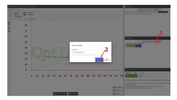
15. Open the "OpenBuild Control". Then, upload the generated G-Code.
