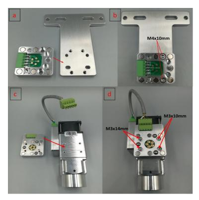
4. Install the LEAD mount (with a relevant element of the docking station) onto the spindle holder. The LEAD mount is designed to be installed on the left, right, or front side of the spindle holder.
