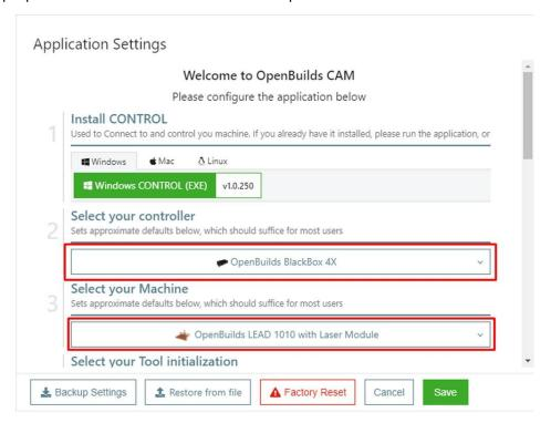
7. In the fourth section of the machine configuration, namely "Tool initialization", select "Turn Laser on and Off: Dynamic Power (M4 / M5)".
