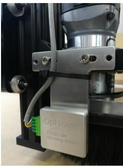
2. Further zip ties can be utilized to fasten the cable at the top of the Z-axis and then along the other side of the X-axis, as shown below:
