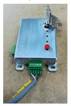
6. Then, connect the LEAD Signal Cable to the output (TOOL HEAD) of the BlackBox controller.
