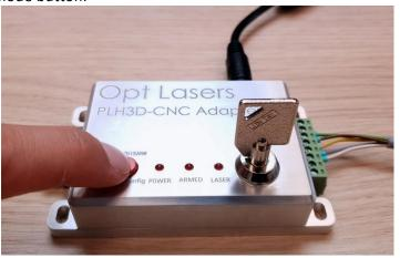
3. Turn the key switch ON while holding the aforementioned button.
