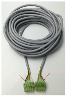
5. Next, connect the laser head cable to the output of the PLH3D-CNC Adapter.
