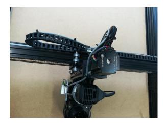
3. Next, secure the cable along the X-axis drag chain using zip ties or by putting it through it.
