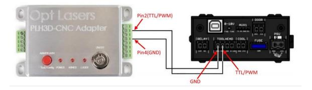
7. Please follow it by connecting the BlackBox signal cable to the input of the PLH3D-CNC Adapter.
