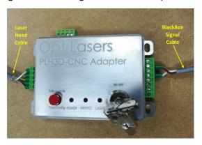
8. Finally, plug the 19 V, 2.5 A desktop power supply into the socket on the PLH3D-CNC Adapter.
